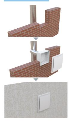
The fan casing is mounted during construction works. Electric wiring for connection of the VNV-1A(E) 80 ventilation unit is led out through a special hole in the casing. The front panel is covered with the protective cardboard plate supplied with the unit to avoid damages or contamination during finishing works in the room. After finishing the works the protective cardboard plate is removed and the VNV-1A(E) 80 ventilation unit is installed into the casing that is connected to the wiring.
